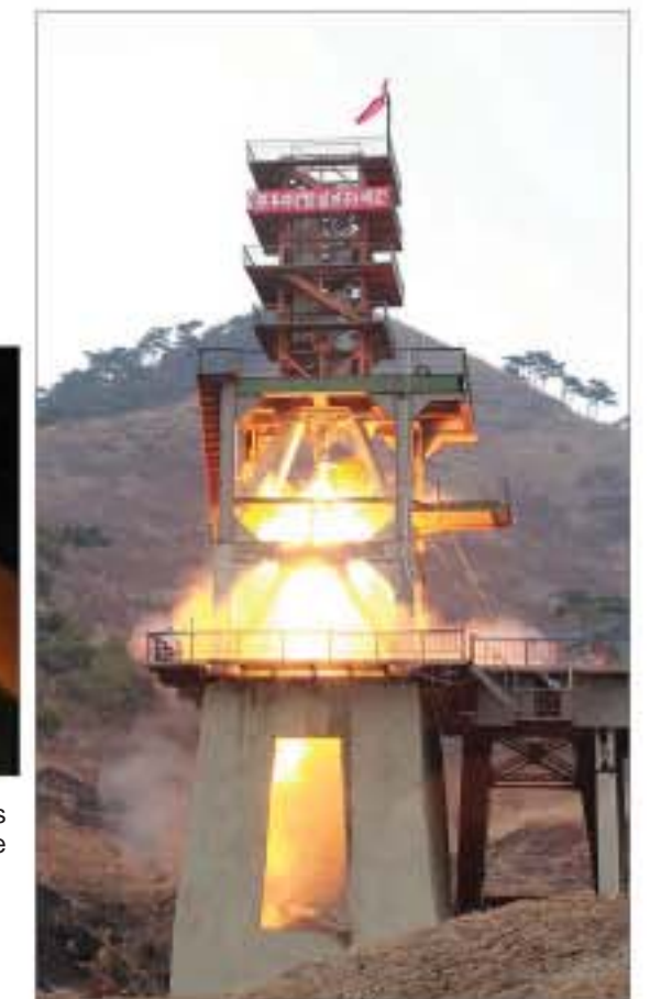
Success in a test that simulates the nose cone tip's re-entry into the earth's atmosphere
