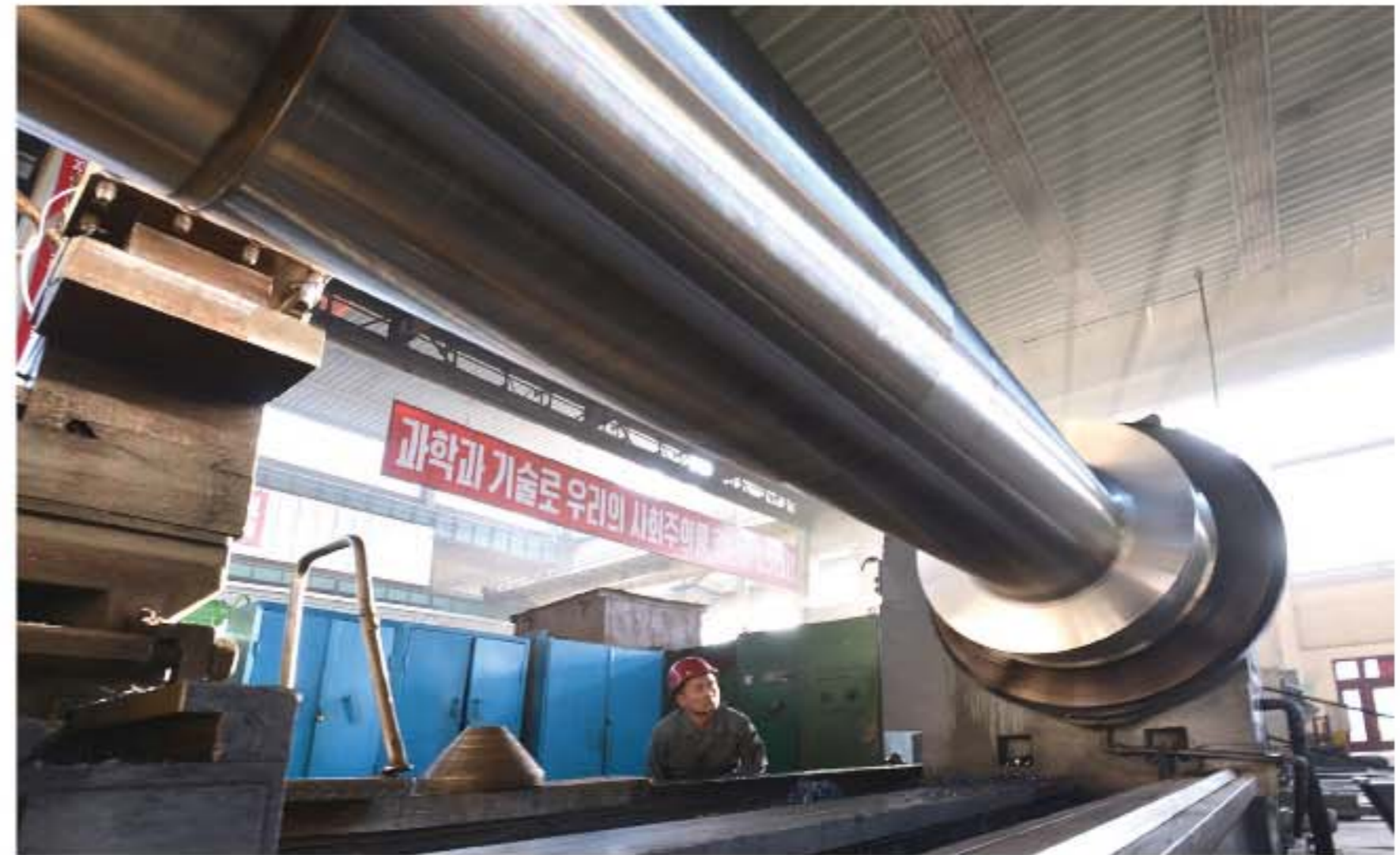
The introduction of CNC technology into a 4-m turning lathe and other large machine tools raises the precision of ordered equipment and electric machines and boosts production
