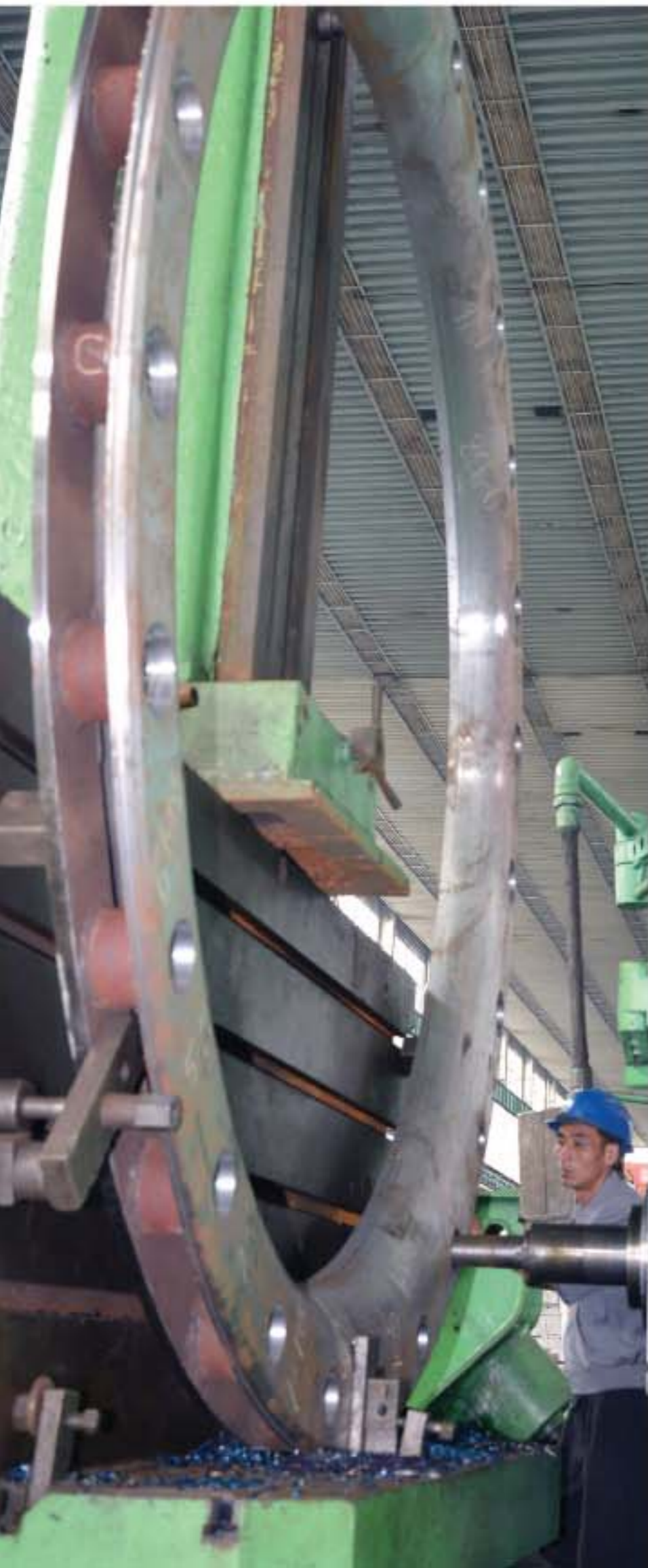
The introduction of CNC technology into a 4-m turning lathe and other large machine tools raises the precision of ordered equipment and electric machines and boosts production
