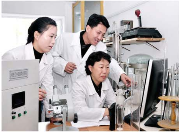
The researchers intensify the research on the technique of measuring the hydration heat of cement.
