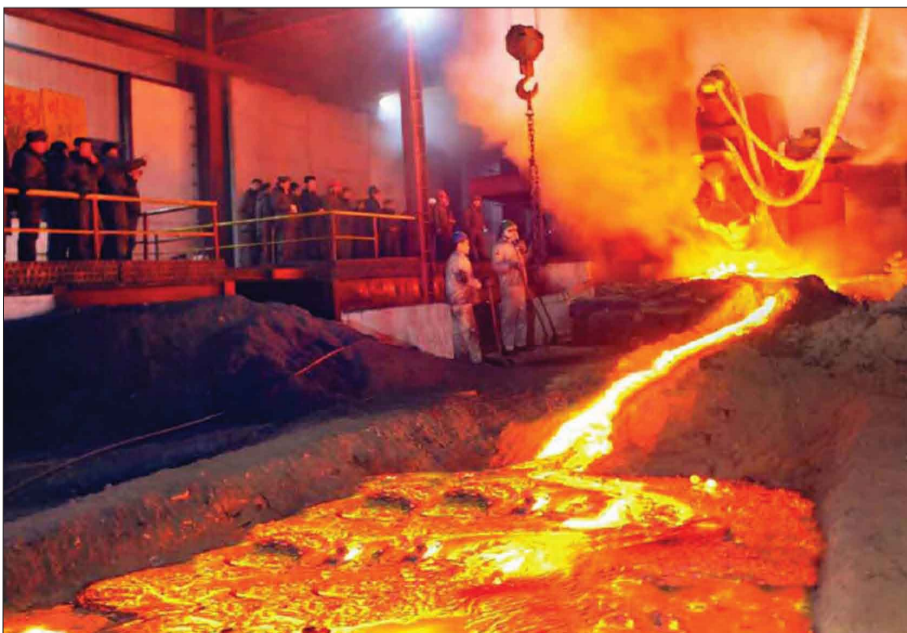
Molten iron is tapped from the oxygen blast furnace at the Kim Chaek Iron and Steel Complex.
