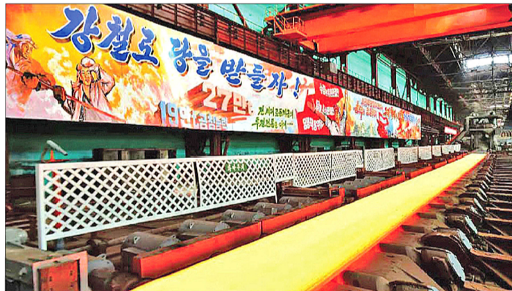
Steel sheets roll off the production line based on coal gasification at the Kim Chaek Iron and Steel Complex.
