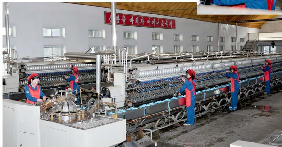
A process of silk thread production from raw cocoons.
