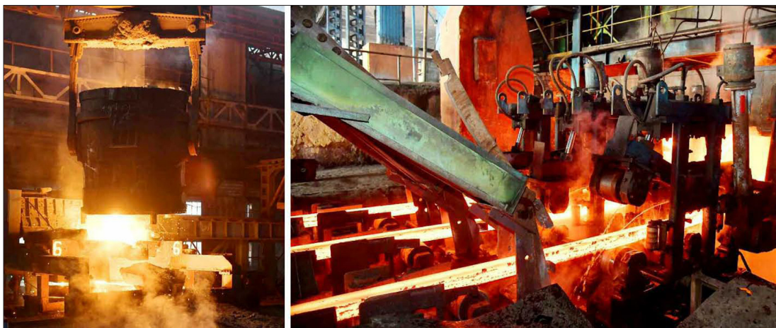
The Chollima Steel Complex in Nampho applies a new jig to reduce the continuous casting process time by two hours and introduces an electromagnetic induction and agitation technique to improve the quality of steel.
