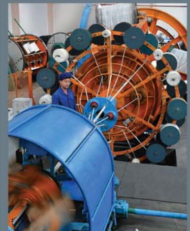
Cabling at Pyongyang General Electric Cable Factory 326
