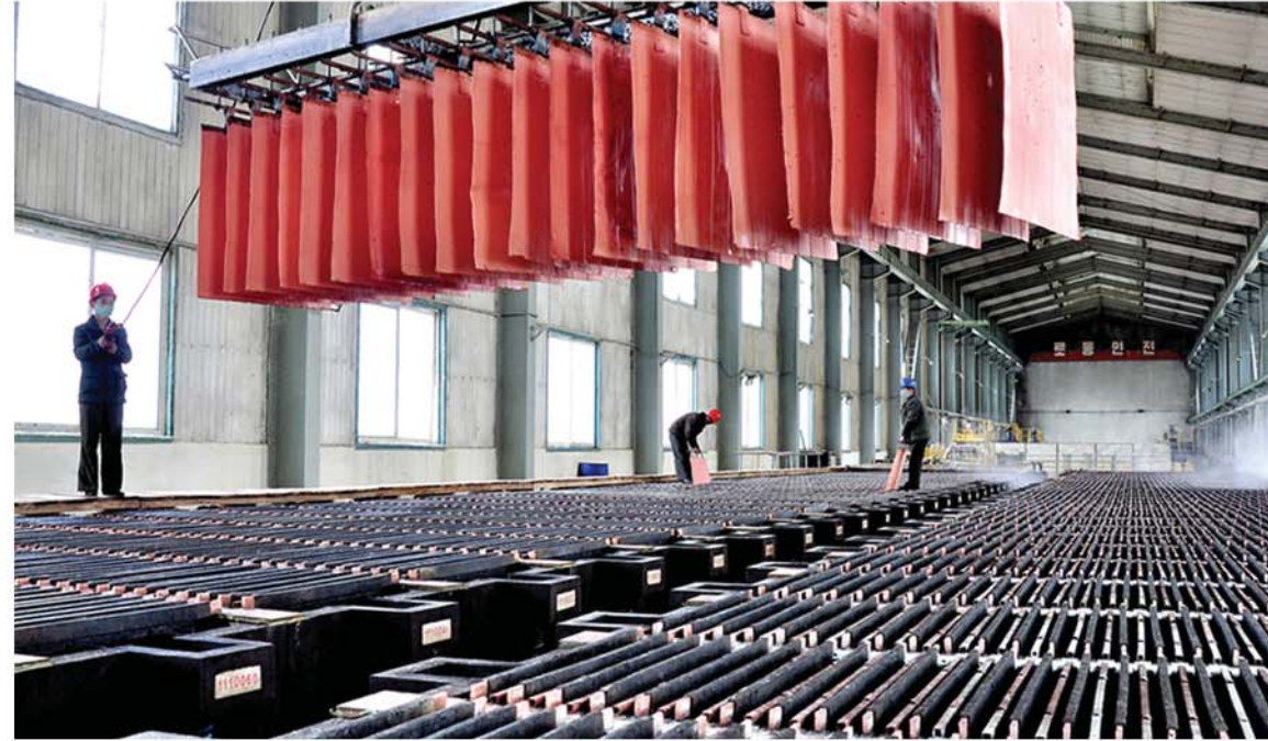
Electrolytic copper production
