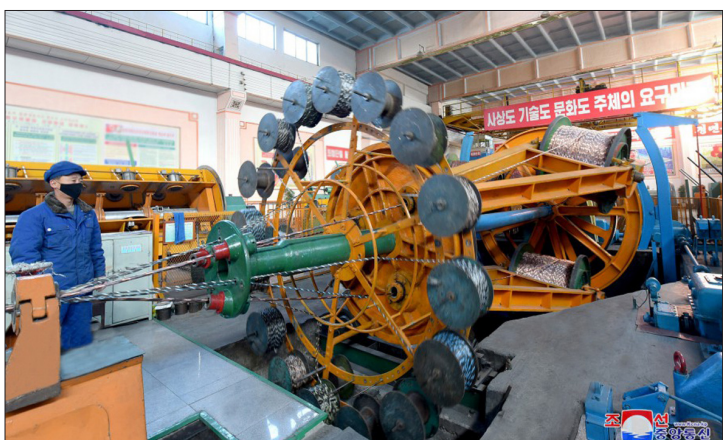
A worker monitors a cable twister at the Pyongyang General Electric Cable Factory 326.
