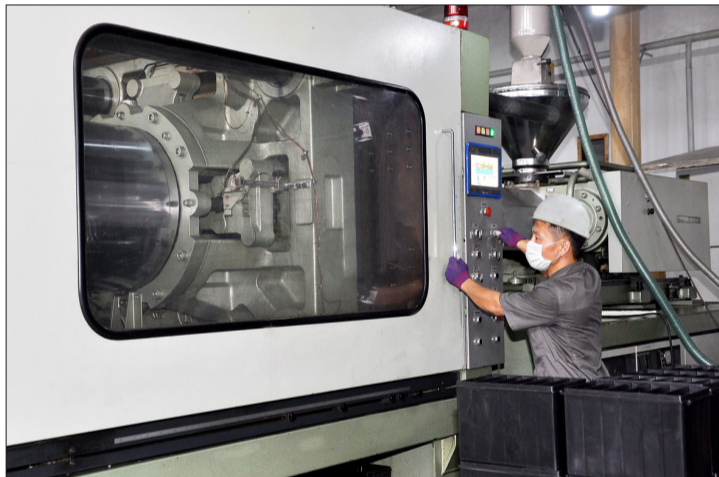
An employee operates the machine to turn out a variety of battery boxes at the Taedonggang Battery Factory.
