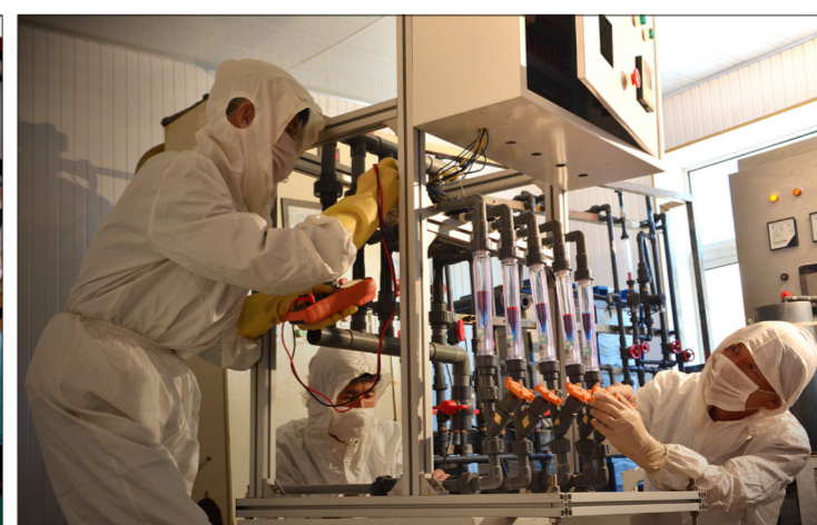
Electronics engineers try to improve the performance of an automatic nutritive solution supply system.
