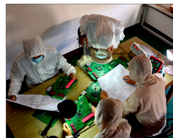
Researchers work on an excitation control device for synchronous generator at the electricity research institute.
