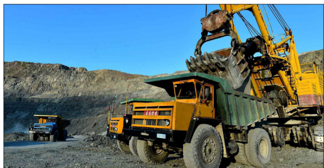
A heavy-duty excavator loads ore on to tipper trucks at the Musan Mining Complex.
