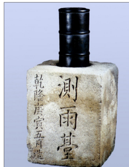
The Koreans made udometer in 1441, the first of its kind in the world.
