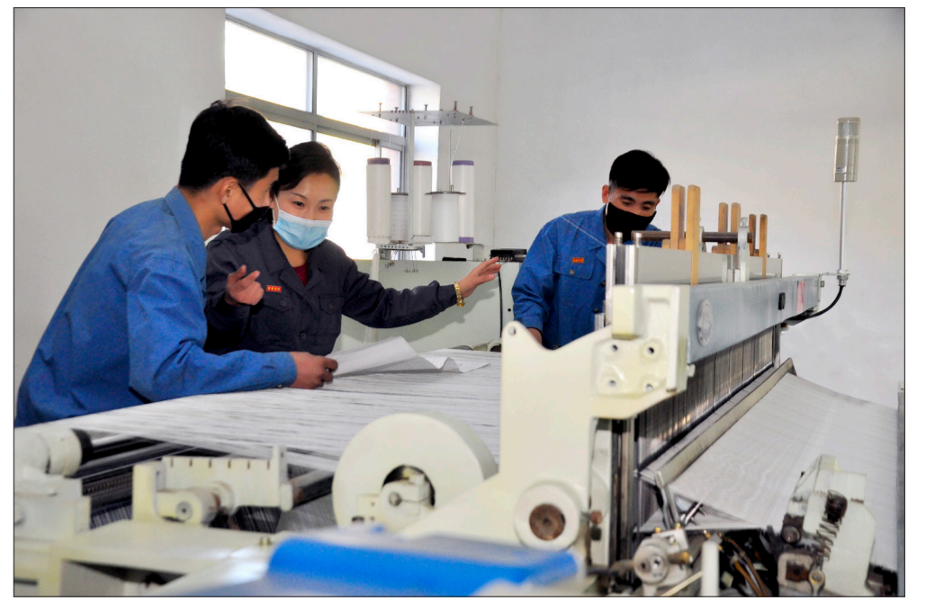
RYU KWANG HYOK / THE PYONGYANG TIMES Technicians discuss how to enhance the performance of a pneumatic jet loom at the Pyongyang Textile Machine Factory.
