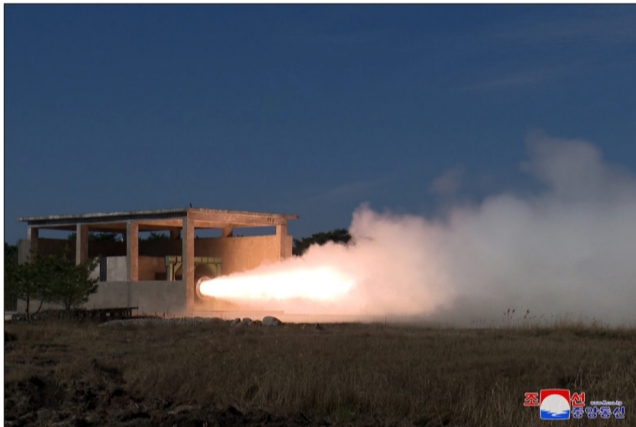
The first static firing tests of the first- and second-stage new-type high-thrust solid-fuel motors for medium-range ballistic missiles are successfully conducted on November 11 and 14.
