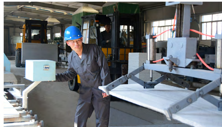
Rough stones produced at the quarry are processed into different kinds of stone works of various sizes, including slabs, railings and kerbs.
